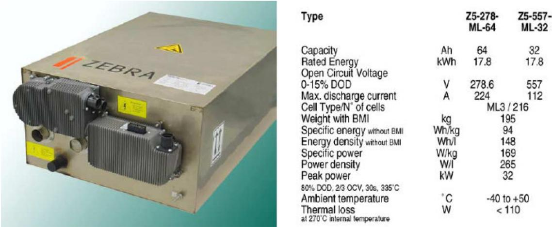
Figure 4. Z5C standard battery with main data
